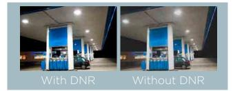
**3D Digital Noise Reduction (3D-DNR)** – Get exceptional video image quality with less noise. 3D-DNR incorporates frame-to-frame noise reduction with spatial noise reduction to produce clear video images with less noise, in low light conditions. Noise reduction is critical for video because noise affects image quality. Cameras with 3D-DNR produce sharper, more accurate video images.
